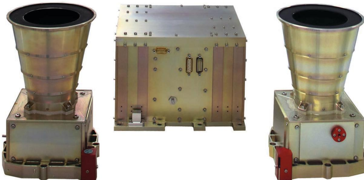
**Unfolding the synergies of star trackers and gyroscopes, ASTROgyro™ establishes a reliable and performant attitude determination system by combining Jena-Optronik's successful ASTRO star tracker series, as source of absolute and drift-free attitude information based on star pattern recognition, with the broad dynamic range and low noise rate spectrum of inertial sensing technology.**
