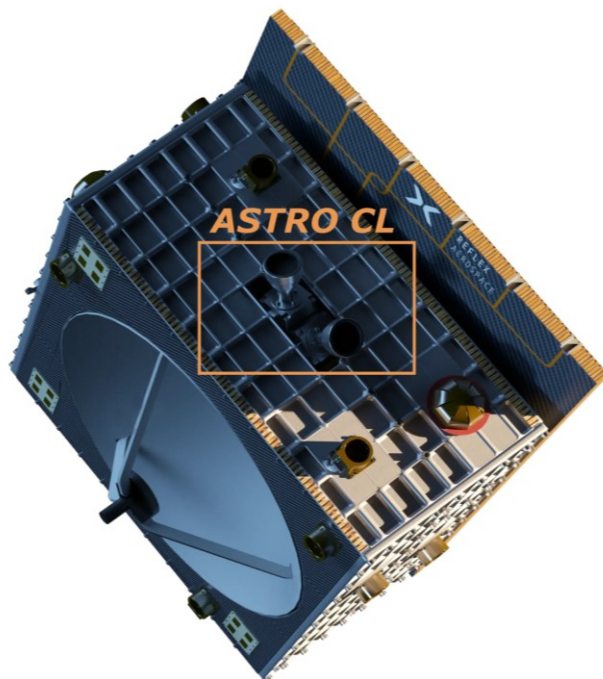
Fig. 2-3: Two ASTRO CLs installed on ReflexAerospace's SIGI smallsat mission (image & info from reflexaerospace.com) to be launched on SpaceX Transporter-12 mission
